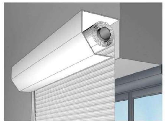
Face fit: Outward roller
